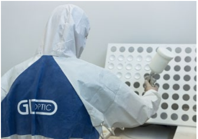
Fig. 6. Painting of integrating spheres with barium sulphate.
